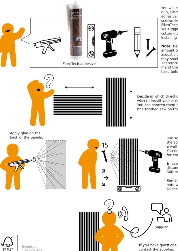
You will need a glue gun, FibroTech assembly adhesive, a spirit level, screwdriver, pencil and FibroTech black screws. We suggest you use cotton gloves when installing your product.
